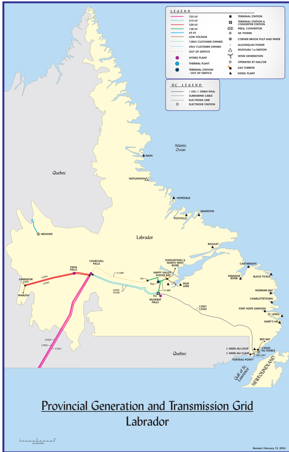
Figure 2 – Labrador Interconnected System
